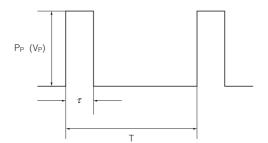
: Pulse limit power (W) : Pulse limit voltage (V) : Pulse continuous time (s)
